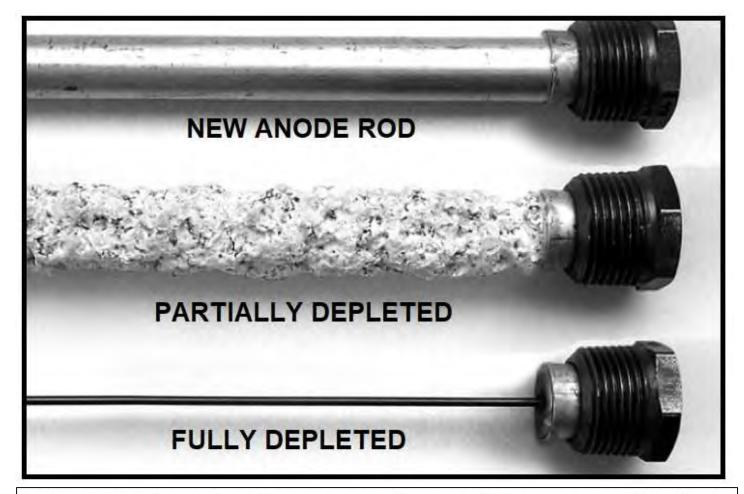
Anode Rod. The anode rod is a sacrificial metal rod that helps reduce corrosion and premature failure (leaks) in the tank. The anode rod is a consumable item.
